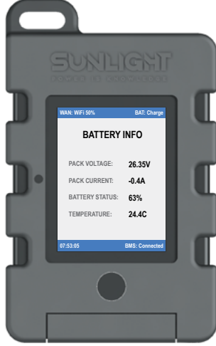
Resim 4 Compact Display Telecommunication Box
